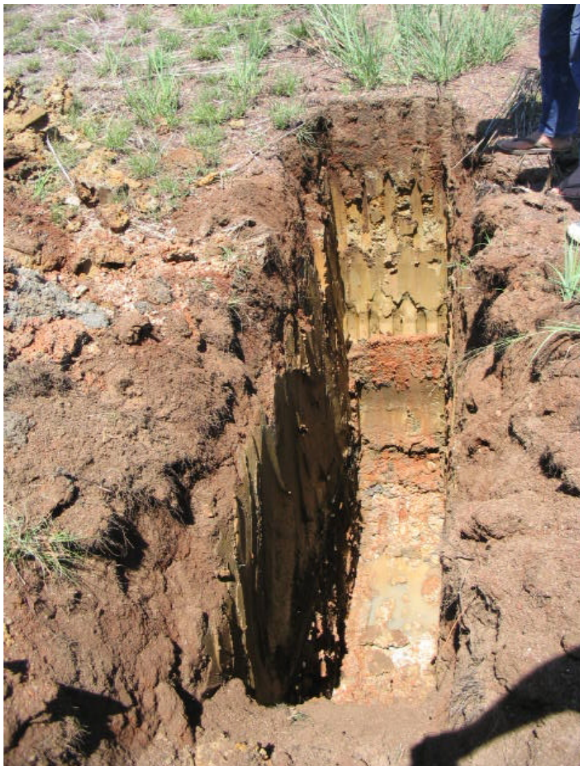
Figure 4 Photo of excavated trench at the Mudla farm showing heavy clay subsoil and sand gravel topsoil (Source : Gwalwa Daraniki Enterprise Pty Ltd ,Mudla farms Mud crab Project,Progress Report 1, December 2005)
